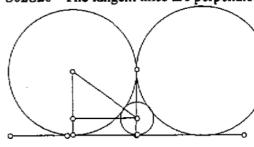
diagram. The hypotenuse is the sum of both circle's radii, r + 5. One leg is the difference between the radii's lengths, r - 5. Therefore  $(r+5)^2 = r^2 + (r-5)^2$  yields r = 0 or r = 20.
